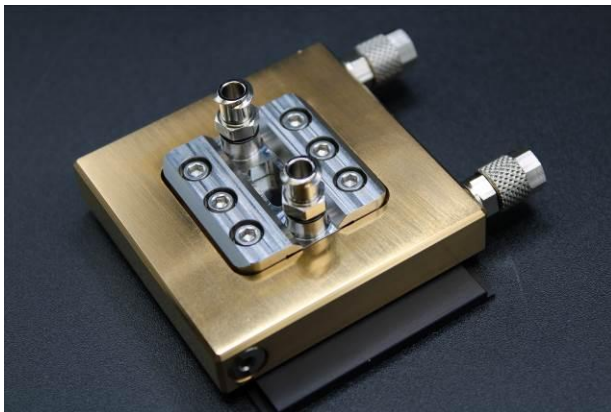
Diamond liquid cell mounted in copper body with cooling/heating channels for temperature control
