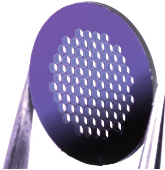
Thin diamond membrane (500 nm) on silicon support grid. Cell size: 800 \mu\text{m} . 78 % open area. 7 mm free aperture
