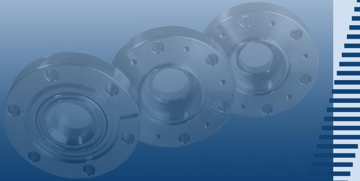
**Diamond Materials** manufactures CVD diamond windows and filters for high-brilliance synchrotron beamlines. Our offer includes water cooled X-ray windows as well as infrared windows with broadband transparency ranging from the visible over the infrared to microwaves. These windows separate the UHV of synchrotron storage rings from the remainder of the beamline.
